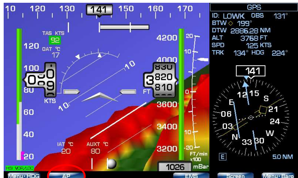
EFIS/GPS screen when Towing Menu is OFF
