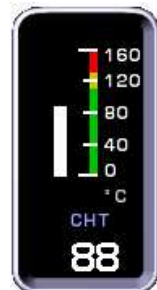
Cylinder Head Temperature (in meaning used by ROTAX, technically the sensor is placed on engine block)
